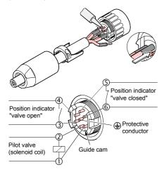
Tighten the strain relief and insert it (it will catch).
